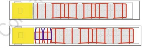
A further check and, if necessary, retensioning of the belts is necessary after special driving situations (evasive manoeuvres, emergency braking or driving through a bad stretch of road).
