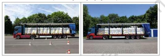
The driving tests carried out on the 25<sup>th</sup> of May of 2012, for the purpose of this report showed that, with an interlocking fit to the end wall and the big bags to each other in combination with appropriate head lashings, safety requirements pursuant to
